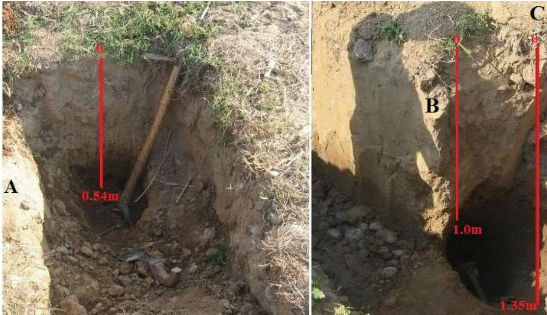
Figure 3: Show the points where the samples were taken below the top of the surface site NGT-2: (A) At 0.54m, (B) at 1.0 m and (C) at 1.35m below the top.
